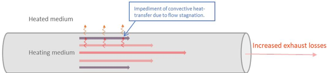
\* Example heat exchanger tube without turbulators.
