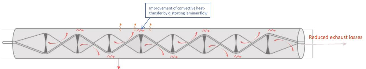
\* Example of heat exchanger tube with turbulators.
